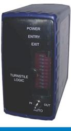
The TL300 is a turnstile logic unit which has been developed to control turnstiles using magnetic solenoid locks and limit switches. The TL300 accepts inputs from card readers or push buttons and performs all of the required timing and interlock logic.
