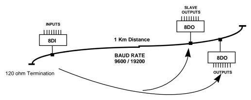
INPUTS ARE SENT TO OUTPUTS AND ALSO SLAVE OUTPUTS
