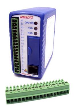
The 8 digital outputs are open collector (NPN). The outputs may be used to drive lamps or external relays when more drive capability is required. The outputs are isolated from the logic and they share a common negative terminal.
