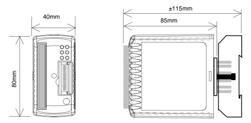
External dimensions of a typical module. Extra space will be required in the front for field wiring.(Approx. 25mm)
