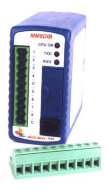
Note: The count values are battery backed-up and will not be lost if power is turned off.
