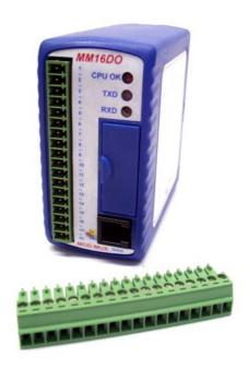
An output watchdog timer can be configured to switch off all the outputs if there has been no communications with the module for up to 255 seconds. A value of 0 seconds will disable this timer and the outputs will remain in the last programmed state.
