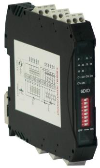
The outputs are written to by the Modbus master device such as a PC or PLC. Each output can be individually switched on or off, or all outputs can be set up at the same time by writing a single number to the output register which represents the status of all outputs.
