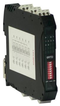
Note: As there is no inter-channel isolation, isolated RTD's must be used in order to prevent ground loops and reading errors.
