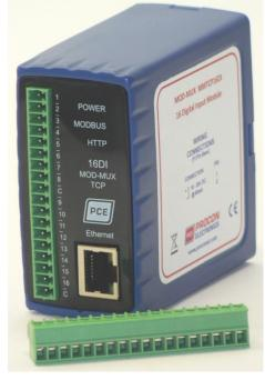
In **mode 2** the inputs are connected as up/down counters. Input 1 will increment counter 1 whilst input 2 decrements counter1. In the same way, inputs 3&4 operate counter 2, inputs 5&6 operate counter 3 and inputs 7&8 operate counter 4.
