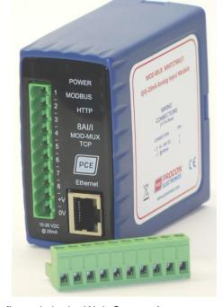
PLC. The IP address in the MMTCP8AI Module is configured via the Web Server. Any standard Web browser such as Internet Explorer can be used to access the web pages were configuration is carried out. The converters are factory programmed with a default IP address of 169.254.111.111. This address must be changed before the converter is added to an existing network.
