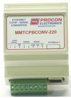
An added advantage of using the converter, is that the Modbus RS485 network can be split into a number of smaller networks, each with a separate converter. This increases throughput dramatically as the single Ethernet network has a much higher bandwidth than the individual RS485 networks and overall data polling times are reduced accordingly.
