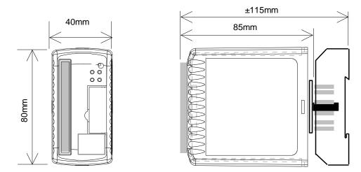
External dimensions of a typical module. Extra space will be required in the front for field wiring.(Approx. 25mm)
