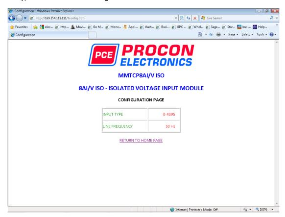
• Input Type: This is the format that the module has been configured to operate with.
