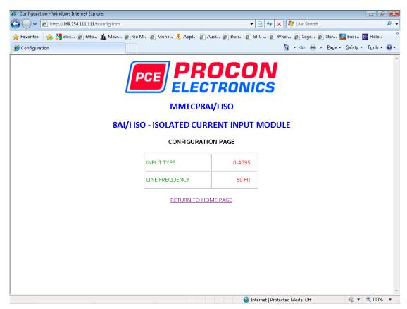
• Input Type: This is the format that the module has been configured to operate with.
